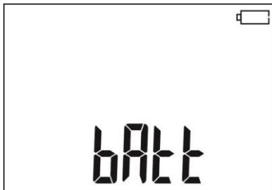
Batteries fully discharged, all measurements are blocked. The meter switches off automatically after 5 sec.
